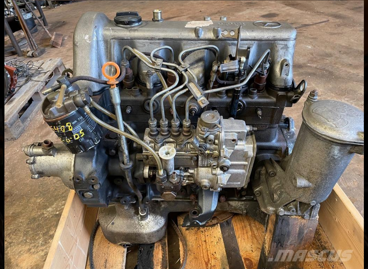
MERCEDES-BENZ OM616 ENGINE (IDI) IDI ENGINE WORK PRESSURE 100-300 BAR
