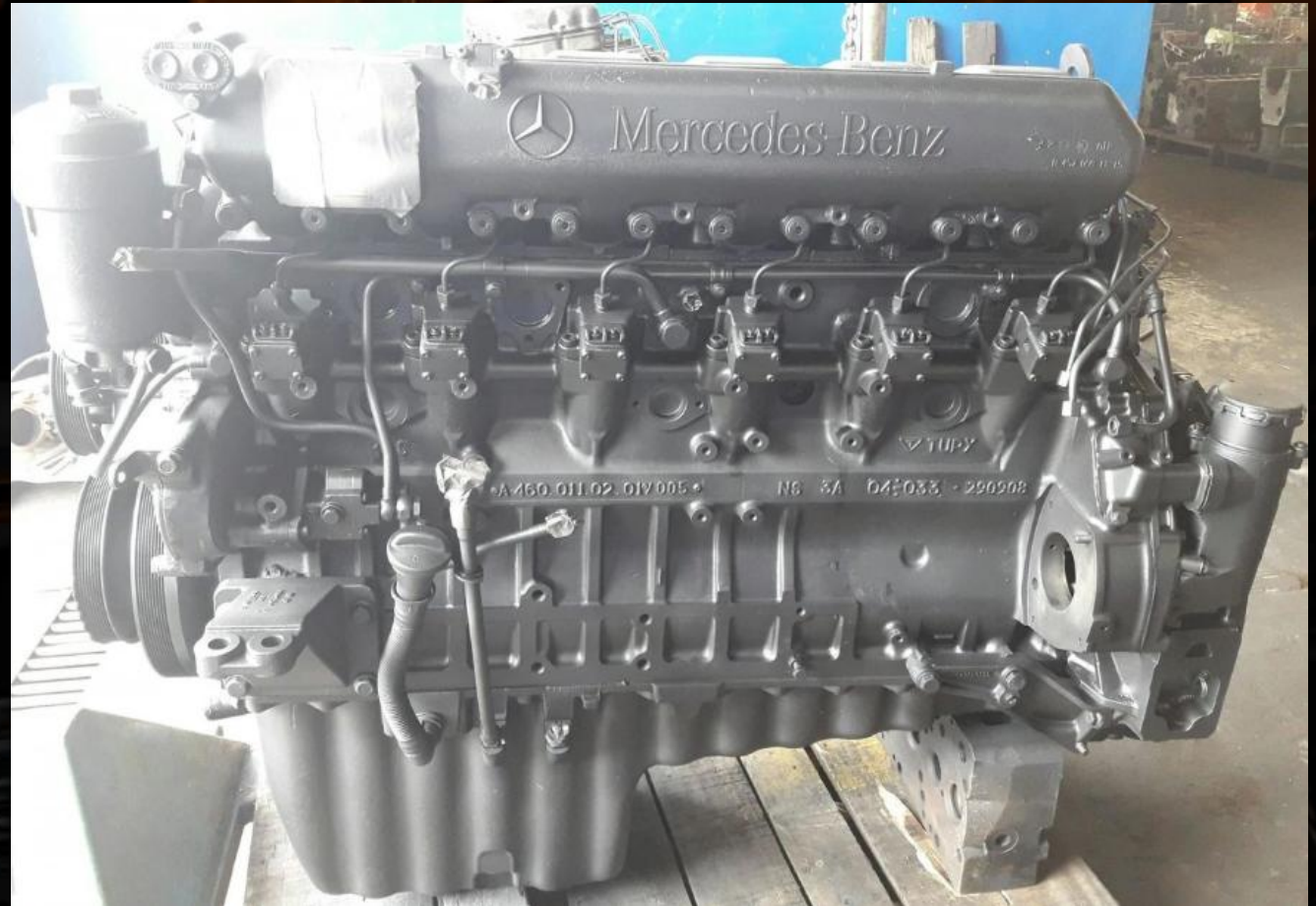
MERCEDES-BENZ OM457LA ENGINE (PD) PD ENGINE WORK PRESSURE 1000-1200 BAR
